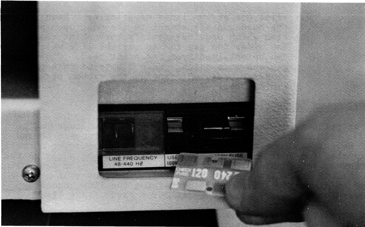
FIGURE 2-4. POWER LINE MODULE
