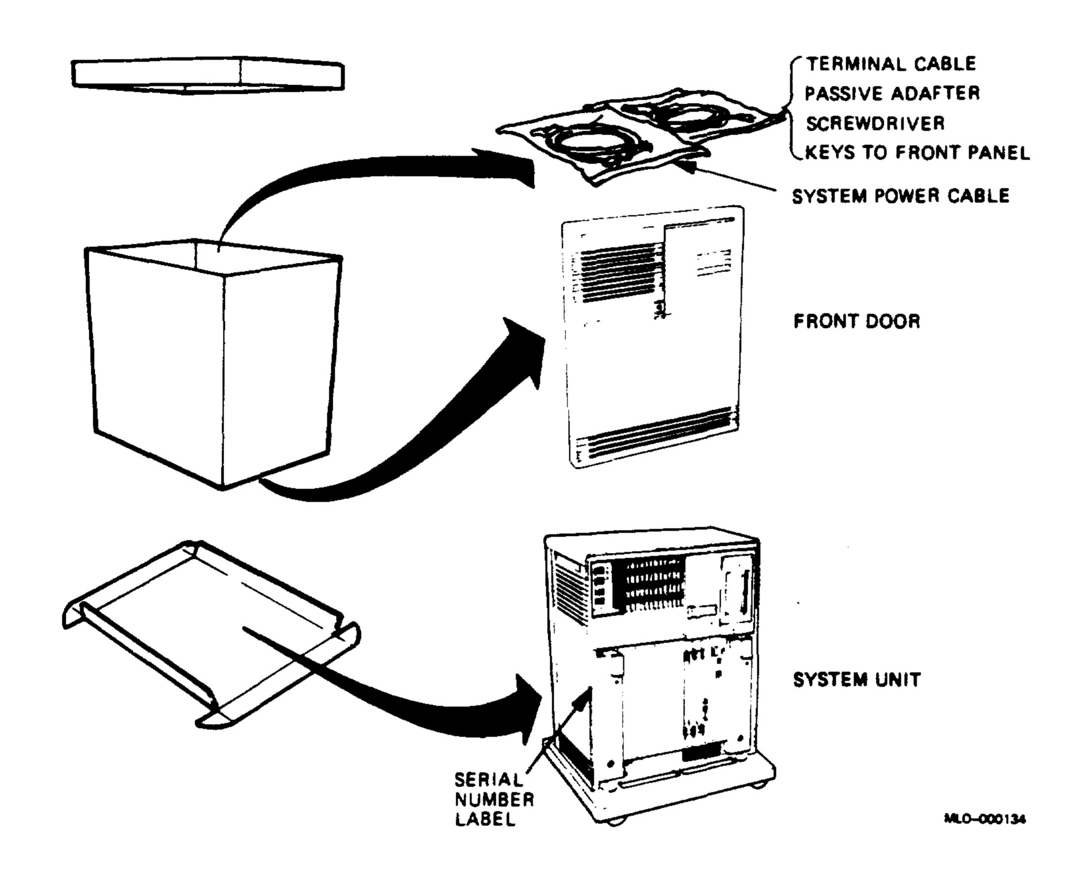
Verify that the system power requirements match the power source. The correct voltage for the system is listed on the serial number label next to the left power supply (Figure 2-2). If the voltage does not match the power source, do not continue. Contact the customer's sales representative.
