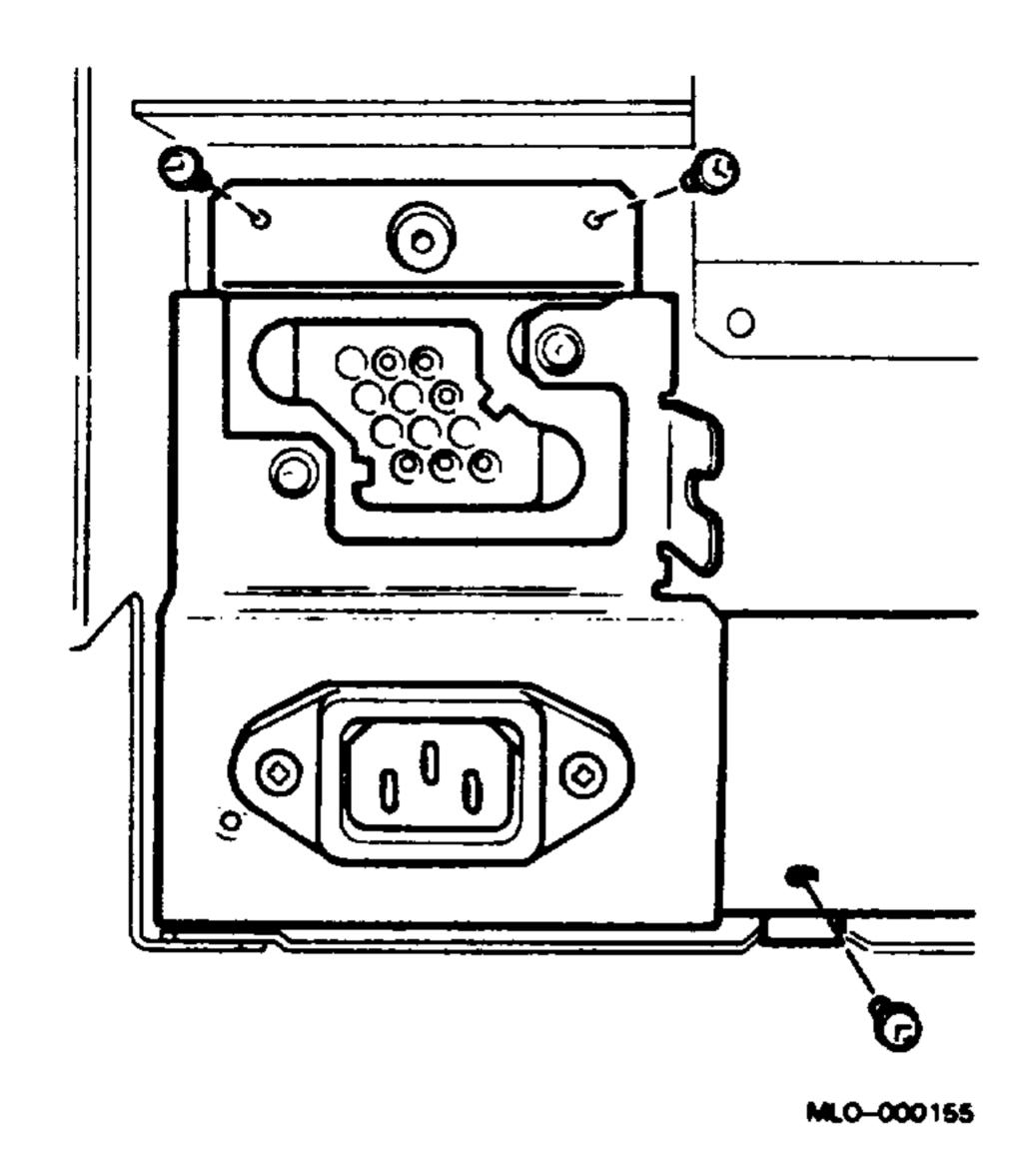
Figure 3–20: Removing the AC Filter
