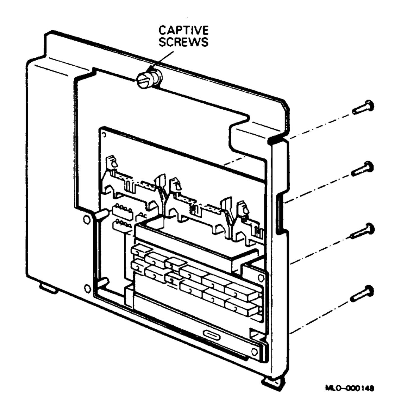
Figure 3-13: Removing the Signal Distribution Board, RD Drives
