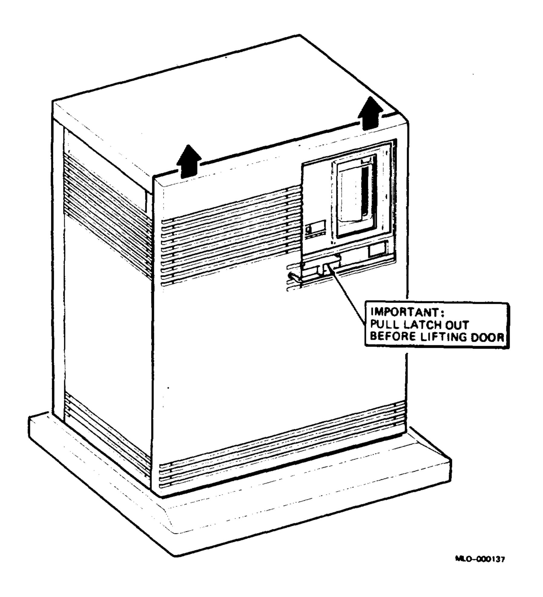
Figure 3–2: Opening the BA213 Front Door (H9644 Cabinet System)
