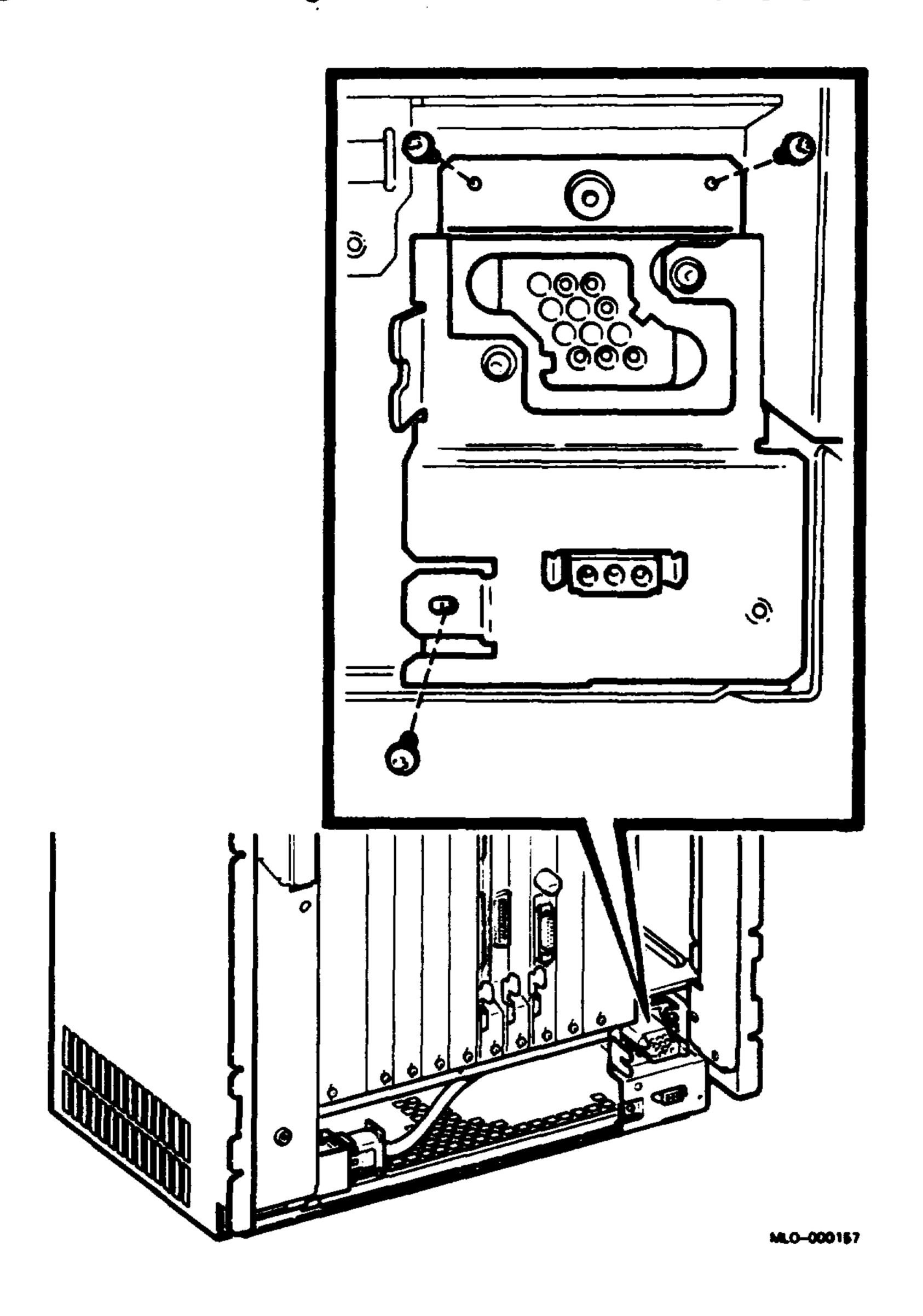
Figure 3–22: Removing the AC Switch Assembly Nuts
