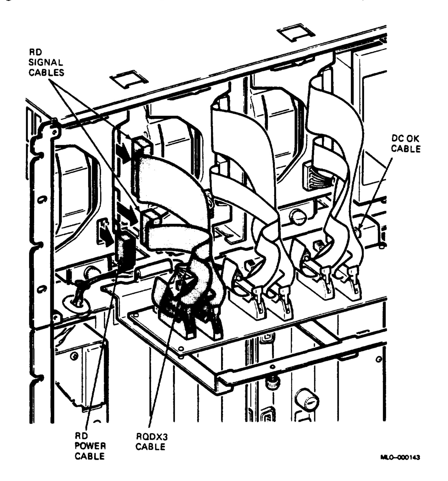
For RD-series drives, the RQDX3 and 10-pin DC OK cables are behind the signal cables on the signal distribution board. Note the orientation of the RQDX3 and DC OK cables, then disconnect the two cables from the board.
