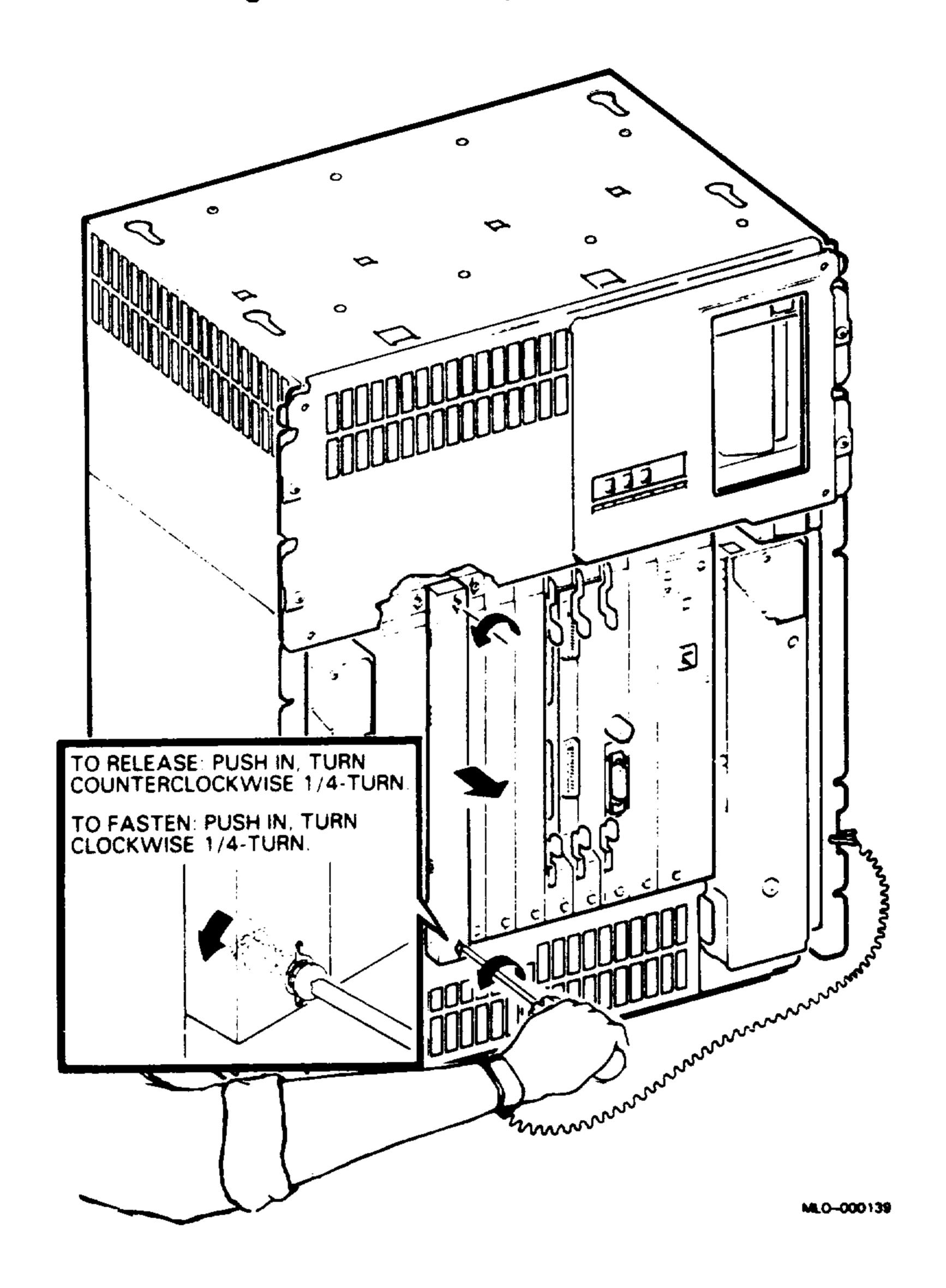
Figure 3-4: Removing a Module
