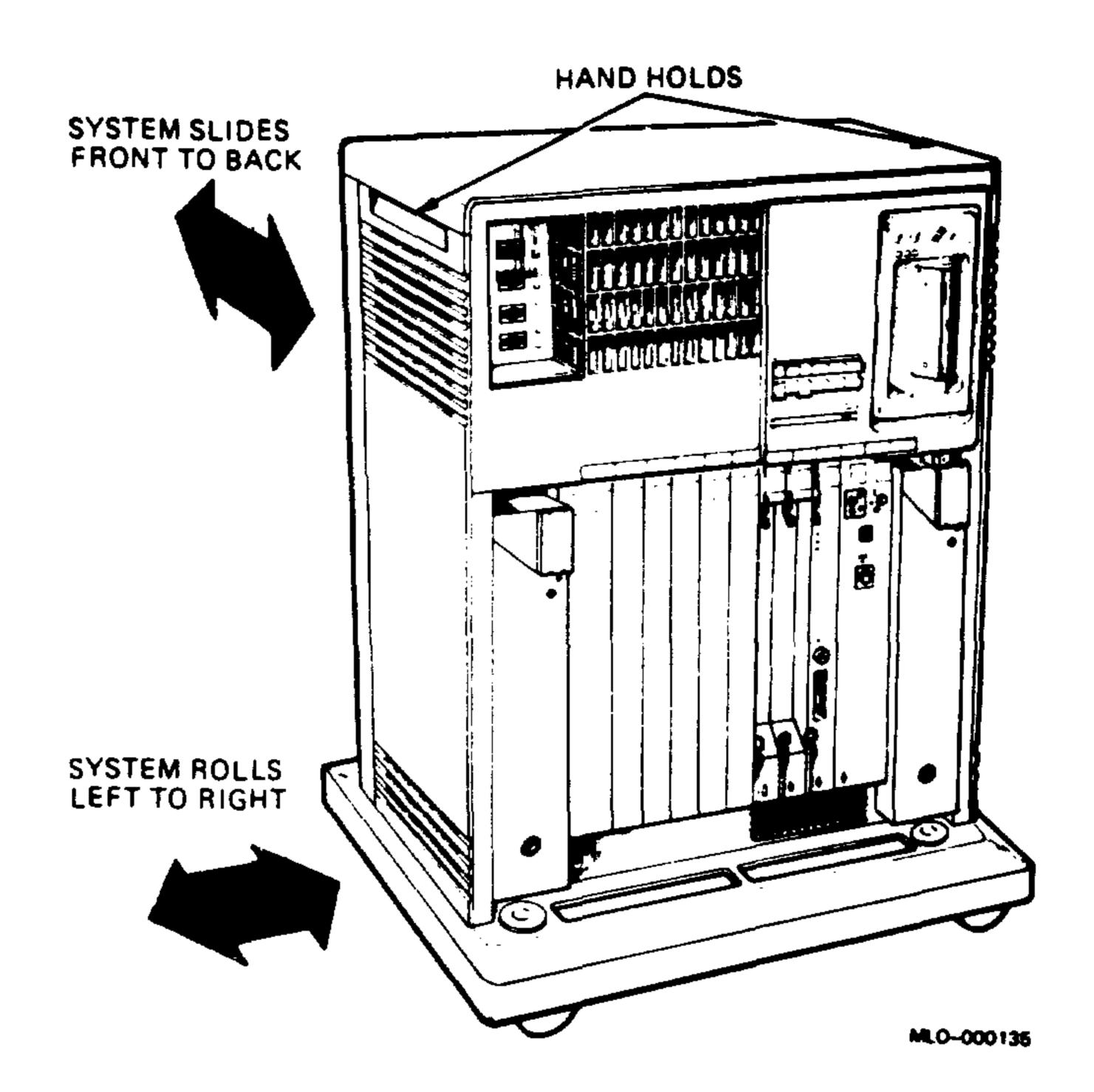
During installation, leave a few inches behind the system for routing cables underneath the system unit. Once installation is complete, you can place the system base directly against a wall.
