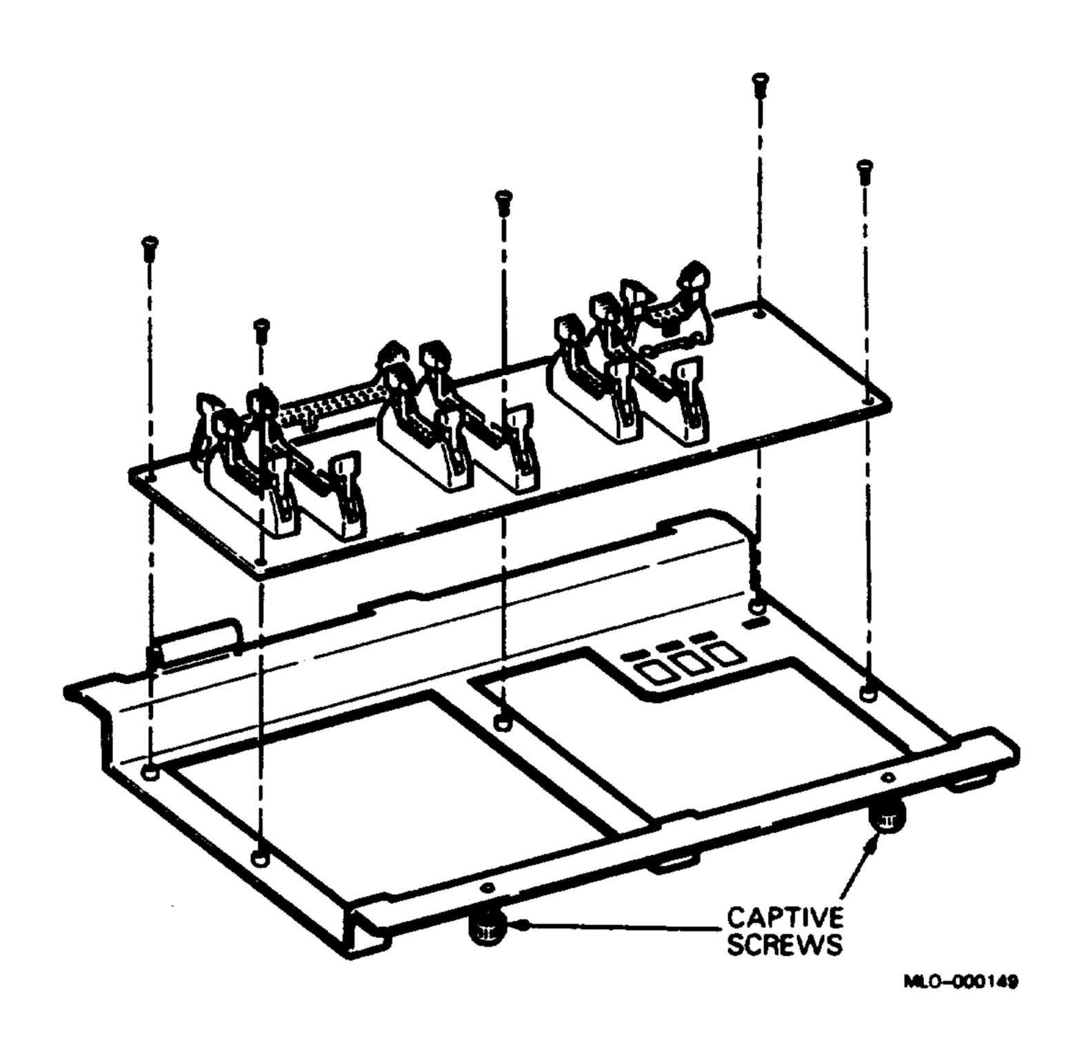
Figure 3–14: Removing the OCP, RF Drives
