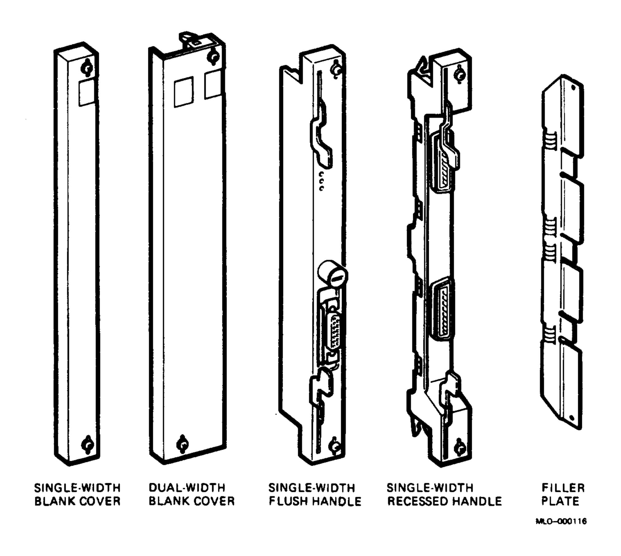
Some modules have special configurations, such as the dual-width panel with I/O connector for the KA630 and KA640 CPUs. Table 1-1 describes common variations.
