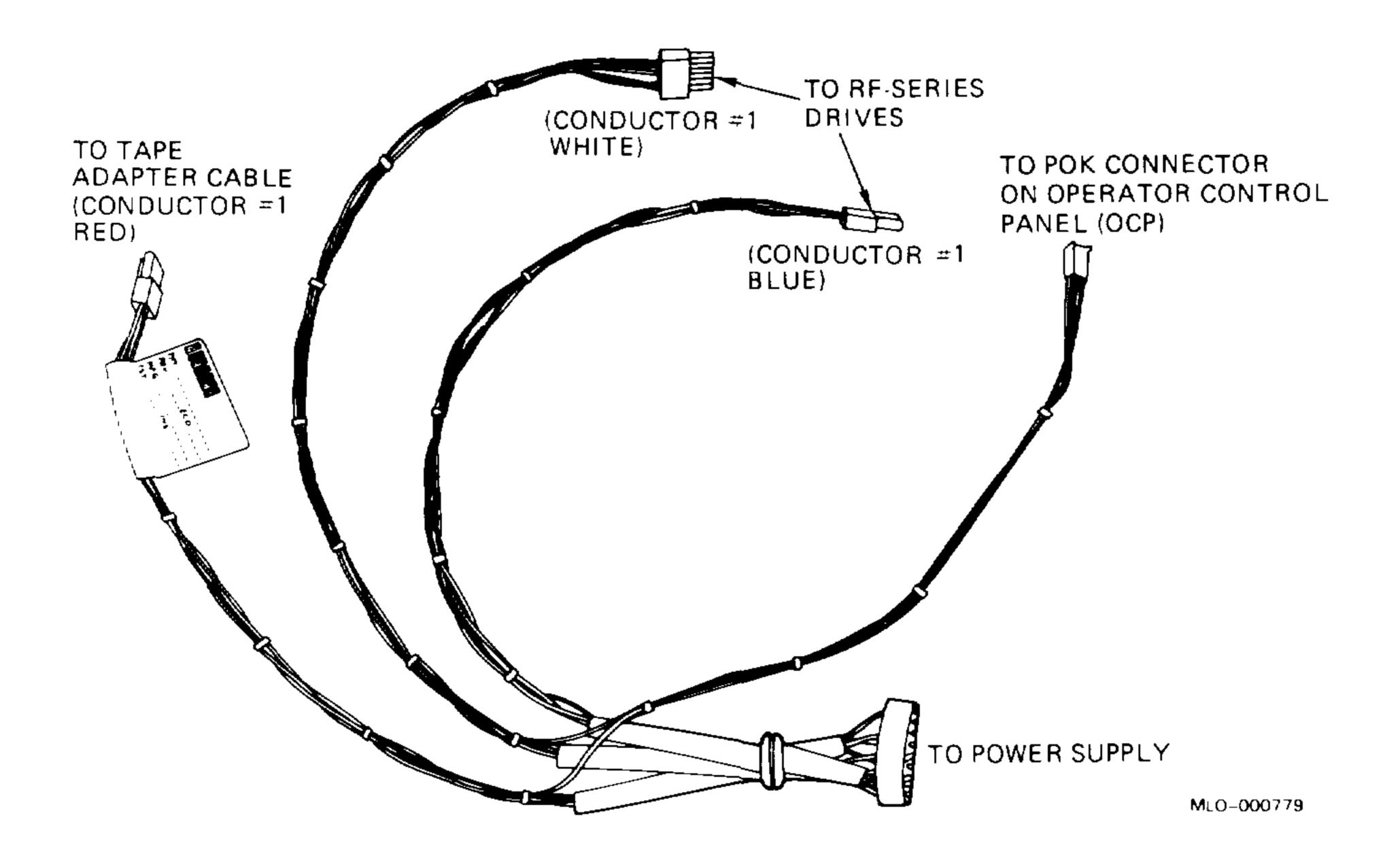
The RF-series OCP contains a three-pin connector for POK lines (color coded) from the power supply (Figure 1–14). The POK signal is on all three lines, and is used to prevent excessive current draw by the disk drives during power-up. The OCP also contains a two-pin POK connector, reserved for future use.
