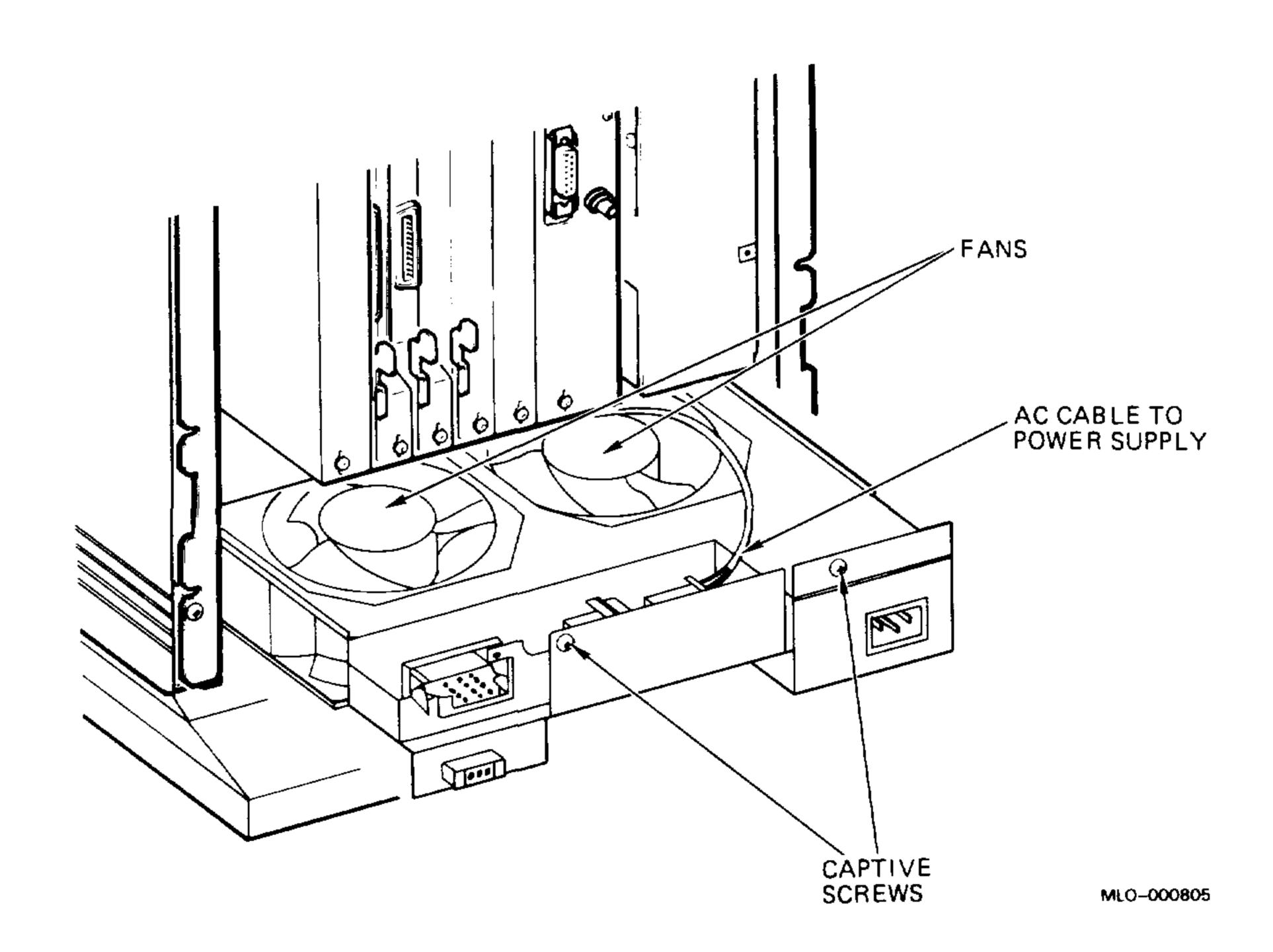
5. Remove the fan tray assembly from the enclosure.
