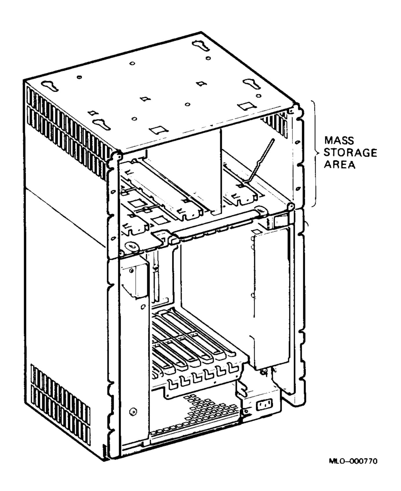
The DSSI supports up to seven storage devices, daisy chained to the host system through either the KA640 CPU or an adapter module such as the KFQSA.
