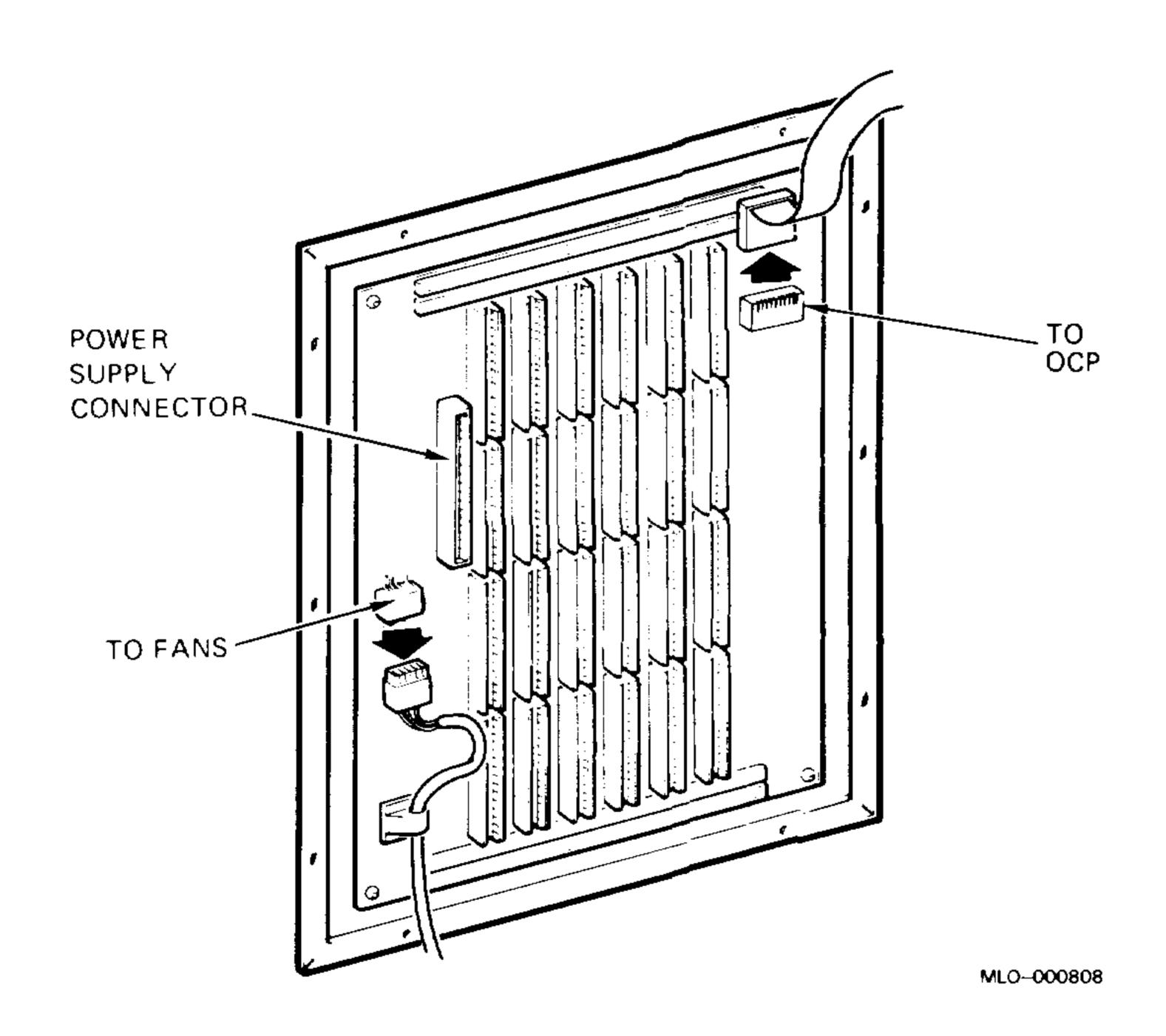
2. Read the Caution below. Then, from the rear of the enclosure, remove the ten Phillips-head screws that hold the metal plate and backplane to the rear of the enclosure (Figure 3–23). The backplane and metal plate are one FRU; do not remove the plate from the backplane.
