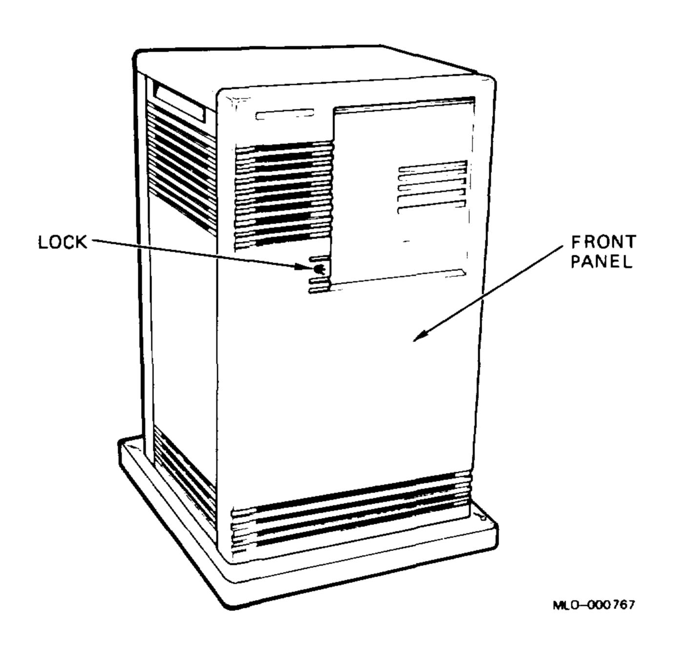
Figure 1–2: BA215 Enclosure Components
