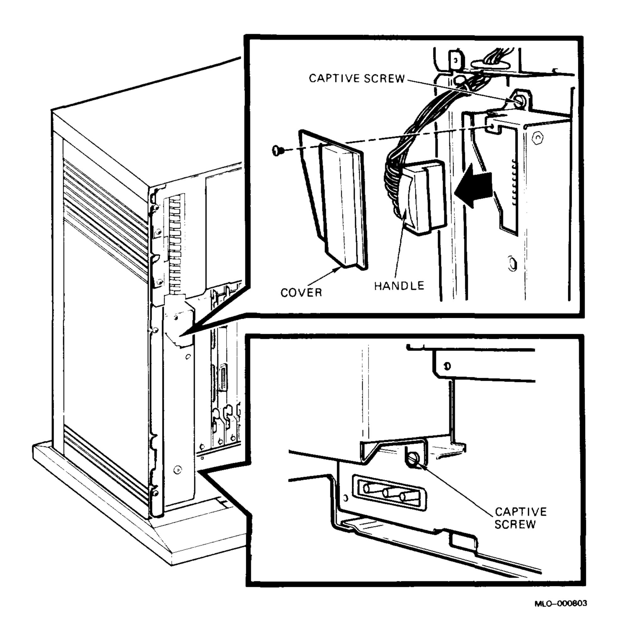
7. The power supply connects directly to the backplane. Remove the power supply by slowly pulling it out of the enclosure, to avoid damage to the backplane connector (Figure 3–18).
