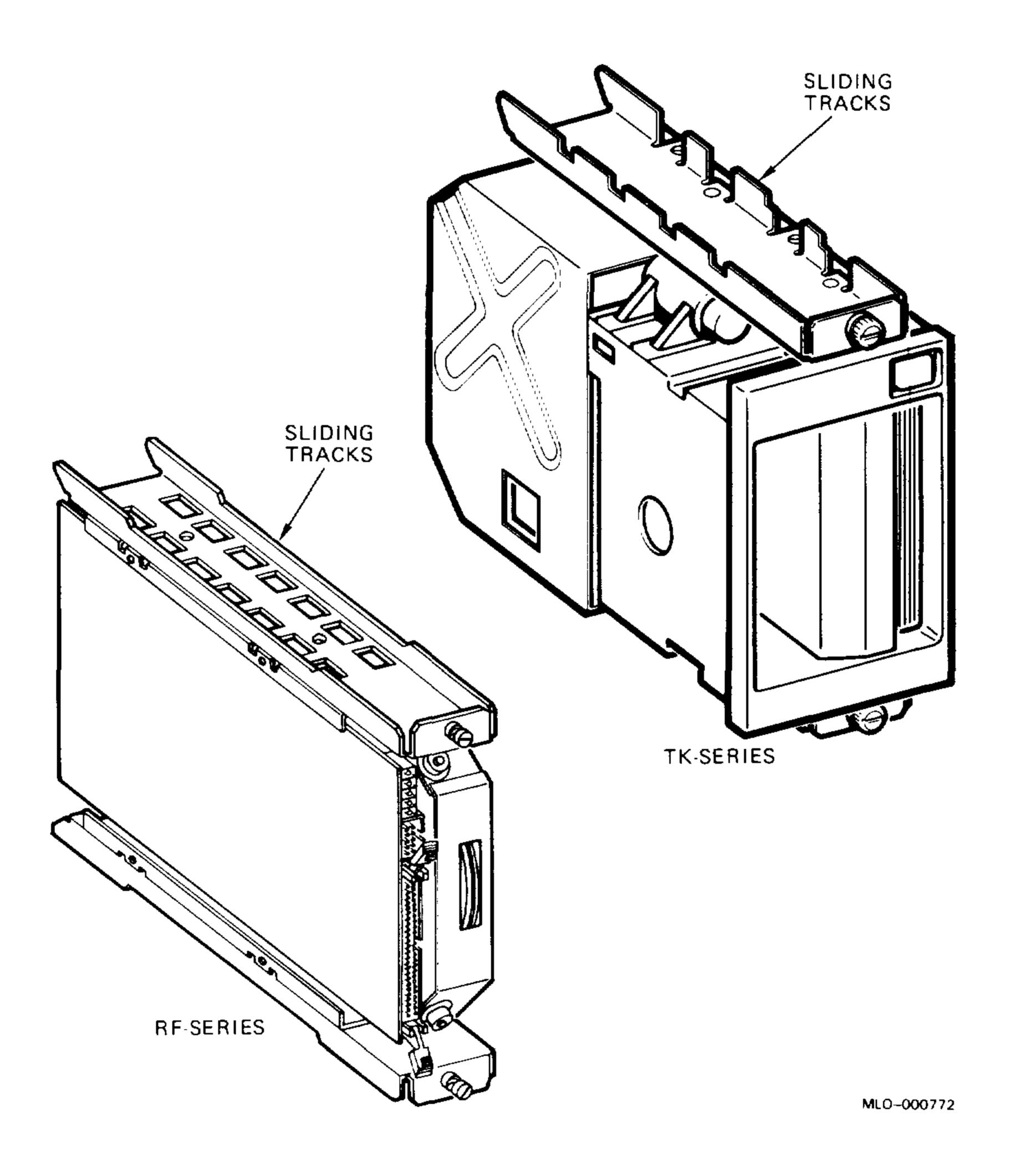
Fixed-disk drives face the rear of the enclosure, providing easy access to drive signal and power cables. TK tape drives face the front of the enclosure, providing access to the controls and tape cartridge opening.
