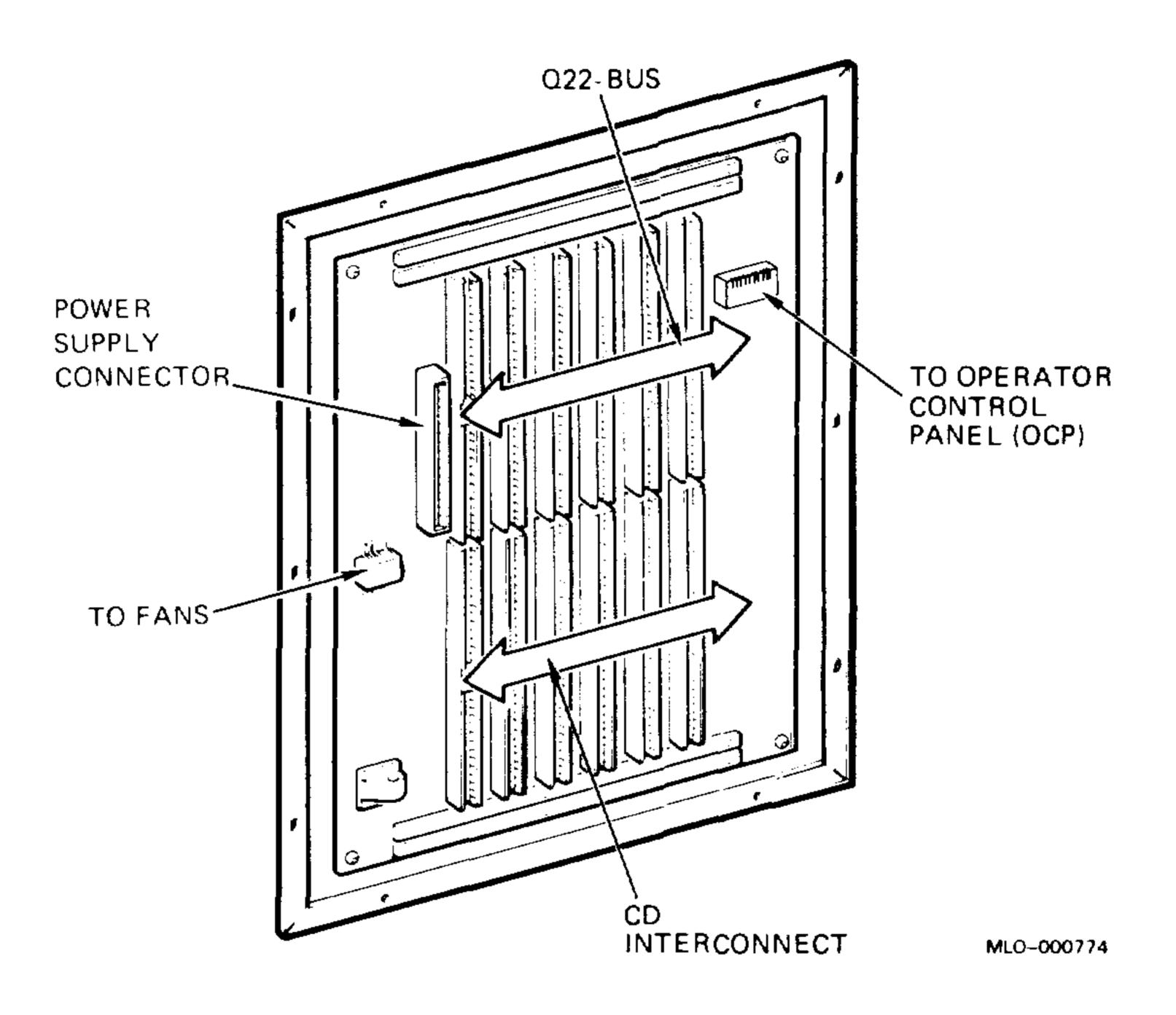
The backplane is bounded and cannot be expanded. It supports 33.5 equivalent ac loads and 20 dc loads. An ac load is the capacitance a module presents to a bus signal line. One ac load equals 9.35 picofarads (pf). A dc load is the dc leakage a module presents to a bus signal line. One dc load is approximately 105 microamperes (µA). The backplane presents 1.5 ac loads to the Q22-bus.
