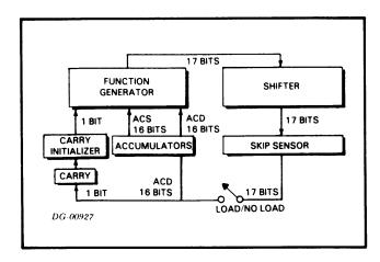
Each instruction specifies two accumulators to supply operands to the function generator, which performs the function specified by bits 5-7 of the instruction. The function generator also produces a carry bit whose value depends upon three quantities: an initial value specified by the instruction, the inputs, and the function performed. The initial value may be derived from the previous value of the carry bit or the instruction may specify an independent value.
