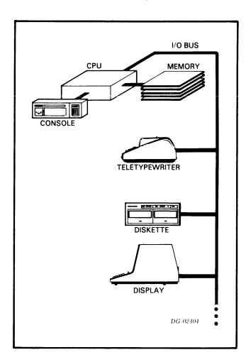
The type, size, and number of memory modules and I/O devices have no effect upon the internal logical structure of the CPU. This chapter deals with the addressing of information and the logical representation of information within the CPU, and is unaffected by those portions of the system outside the CPU.
