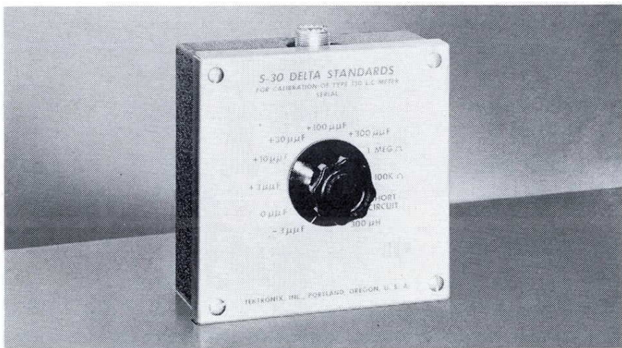
S30 Delta Standards, for calibration of the Type 130 L,C Meter. The unit provides accurately adjusted steps of capacitance and inductance, selected by a rotary selector switch. Values of the capacitance steps correspond to the full-scale adjustments required on the five scales of the Type 130. Two resistors of identical manufacture and similar capacitance, values of 1 megohm and 0.1 megohm, are provided for the resistance compensation adjustment. A 300- \mu h standard permits proper adjustments of the inductance ranges. . . . . 22.00
