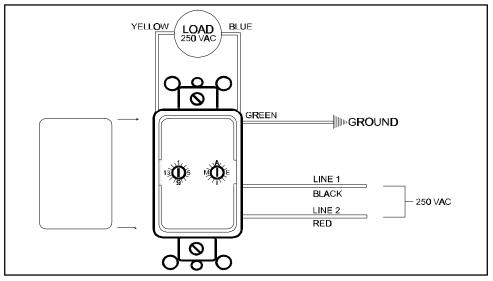
The XPS2 Double Pole (240VAC), 20A Wall Switch is designed for controlling pumps, air conditioners and 2Hp motors.
