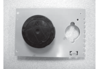
A5180/A5190: Photoelectric Detector Board
