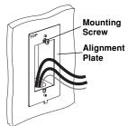
**Alignment Plate Held By Wires**
