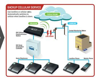
When the C3 is connected to the GSM cellular network, attached telephones can be used to make calls. If a landline is present, you will hear the normal dial tone and you can make your call as normal using the landline service. However, if the landline is currently unavailable, you will hear a different tone which indicates the C3 is in cellular mode and the call will be made using the cellular network. If the landline is available,
