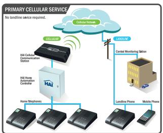
The C3 allows any existing security panel to communicate alarm conditions using the GSM cellular network. The C3 checks the status of the existing PSTN telephone line and if it is unavailable, the C3 will emulate the line signal to the security panel. When an alarm occurs, the security panel will dial out using the GSM cellular network to communicate with
