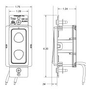
The CA5100 Accessory Wall Switch Controller is a Z-Wave™ enabled device which is fully compatible with any Z-Wave enabled network. Z-Wave enabled devices display the Z-Wave logo and guarantee connectivity and interoperability between devices. Each line powered node in a Z-Wave network is designed to act as a repeater forming a mesh network eliminating radio "dead spots" and providing the highest level of reliability.
