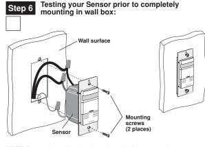
NOTE: Dress wires with a bend as shown in diagram to relieve stress when mounting device.
