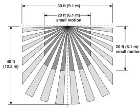
**Small Motion** = Dual Technology coverage. This also represents the maximum ultrasonic range coverage.
