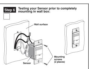
NOTE: Dress wires with a bend as shown in diagram to relieve stress when mounting device.
