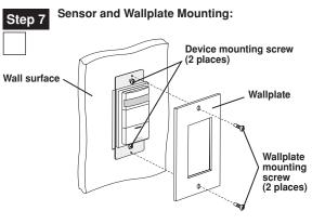
Secure device by firmly tightening mounting screws. Install Decora<sup>®</sup> style wallplate (sold separately).
