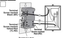
Use Terminal for 3-Way or More Applications Only. For Single-Pole Applications, Do Not Remove This
