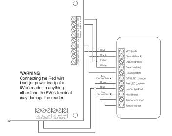
Normal Closed Tamper Connection connect to zone (optional)
