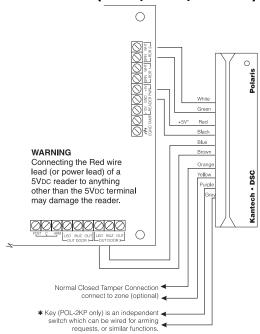
\*NOTE: Only use the +5V power supply when using Polaris Readers.
