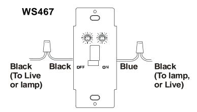
The WS467 Wall Dimmer Module is designed to control **incandescent only** lights with a rating of between 40W and 500W. Lights rated below 40W might flicker or operate erratically. The WS467 replaces a switch that controls and indoor or outdoor ceiling light. A push-button is provided for local on/off control.
