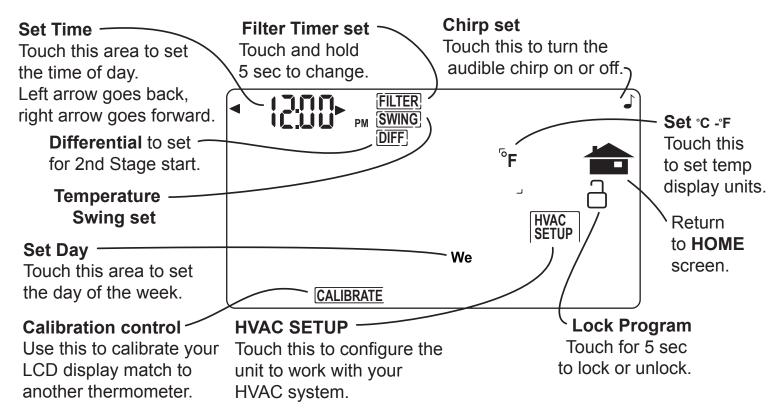
PROGRAM Screen The PROGRAM screen sets the CT30 control for your home HVAC system. It is displayed when you press the PROG button. [See page 7 for details]
